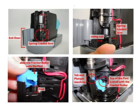
Step 1: Remove the Main Scanner Cover. Open the Exit Door located at the rear of the scanner. Locate the Spring Loaded Arm.
