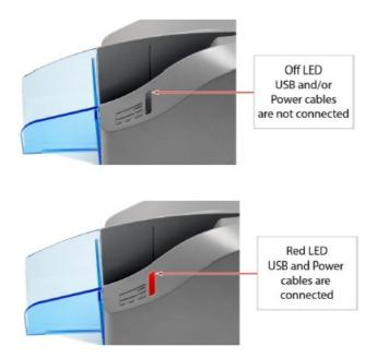
**Note:** Both ends of the 'USB' cable must be plugged in for the LED light to turn 'Red'. If the LED does not turn 'Red', check and reseat the end of the 'USB' cable going into the PC and into the scanner and that the PC is turned on. Then, check that the 'Power Supply' cables are connected properly and the source is live.
