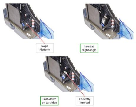
• Step 4: Replace the center cover by setting it back on the unit vertically. Make sure that both sides of the 'Locking Tabs' are fully latched. If replacing an existing cartridge, remove the ink cartridge by grasping the small tab at the rear end and gently pulling upward. Replace the ink cartridge using the steps above.
