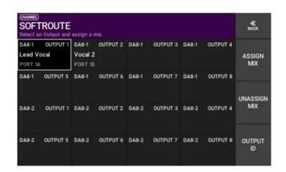
**NOTE:** Softroute can easily switch between mixes and outputs. For example, someone may have a guitar mix on a Livemix Pro DUO Mix A and a keyboard mix on Mix B. With Softroute, the mix sent to a wireless transmitter can be switched seamlessly. The same performer can get a guitar mix switched to a keys mix remotely.
