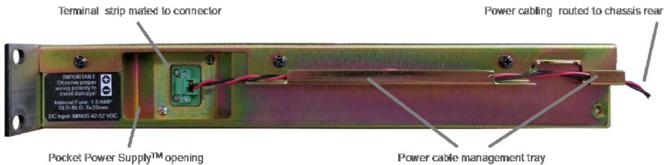
Figure 7: R232-48VDC side view with DC power cabling installed and properly configured.
