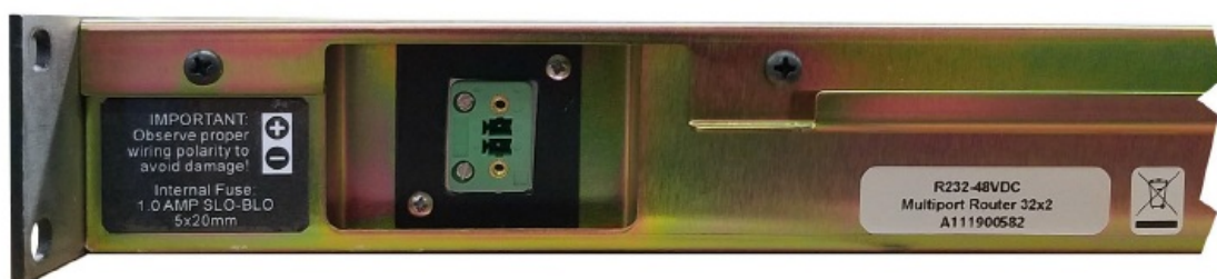
Figure 6: R232-48VDC Pocket Power Supply with removeable terminal receptacle for DC input (shown with mating connector removed)
