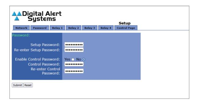
If the passwords are forgotten, the R198 can be set back to factory defaults by removing the power from the unit, pressing and holding, the Reset button on the back of the unit, and reconnecting the power to the unit while keeping the button depressed. After approximately 10 seconds you can release the Reset button and the unit will be reset to the default password of 'digital' for Setup and no password for Control.
