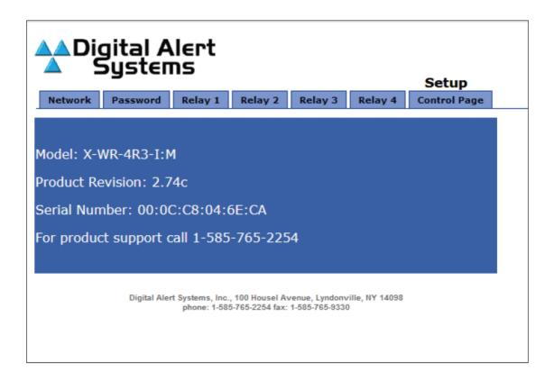
**Setup Configuration:** Setup mode of the R198 allows you to customize several settings. Some of the settings are the unit's IP address, Netmask, Gateway, network speed, mode, and passwords. No username required to log into the Setup, and the default password is shown in bold between the quotes 'digital'.
