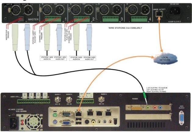
100 to 240 VAC power is input from the universal line in connection. The local ethernet cable RJ45 connector is plugged into the LAN socket. The audio input is switched into the AES card, converted to an AES digital stream, and substituted for the program digital stream via software command over the ethernet link from the DASDEC EAS Controller.
