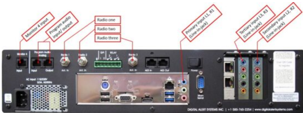
Back Panel View shown with optional EXP-2NICGIG and EXP-EAS monitoring audio expansion
