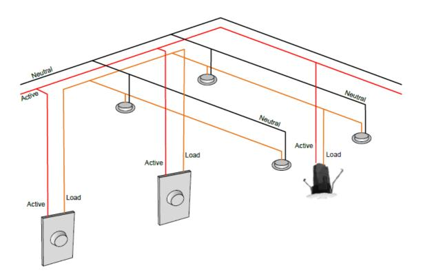
When connected in parallel, LEDsmart+ dimmers, timers, switches and occupancy sensors allow dimming and switching of connected lighting loads from multiple locations without any additional wiring. No strapper wires, dedicated remote switch wiring or control bus is required.
