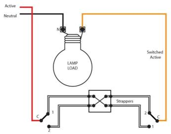
Traditional three-way switching using two rocker switches and one intermediate switch, with stripers between the switches.
