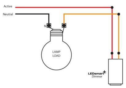
Replacing existing one-way switch with one-way switching/dimming
