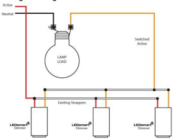
Rocker switches and intermediate switch replaced with LEDsmart+ dimmers. The existing stripers are used to connect the dimmers in parallel. No new wiring is required.
