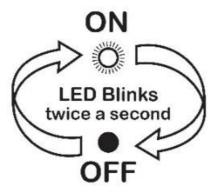
**Step 3** The dimmer is ready for the settings to be adjusted as required. Go to the relevant setup function instructions
