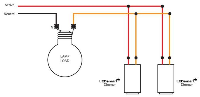
Two-way dimming and switching using LEDsmart+ dimmers. Note the two-wire dimmers are simply wired in parallel.
