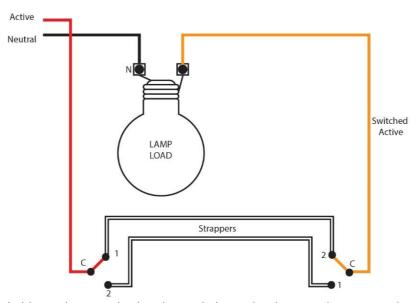
Traditional two-way switching using standard rocker switch mechanisms and scrappers between the switches.
