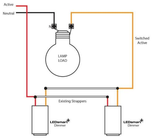
Rocker switches replaced with LEDsmart+ dimmers using the existing strapped wires. No new wiring required.
