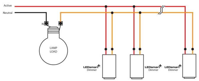
Three-way dimming and switching using LED smart+ dimmers. Note that each two-wire LED smart+ dimmer is simply wired in parallel.
