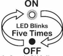
**Step 4** To set Indicator to glow on when the dimmer is off (default) Push and hold the button to adjust the level until the lamp(s) turn ON To set the Indicator to turn off when the dimmer is off Push and hold the button to adjust the level until the lamp(s) turn OFF **Note:** To cancel/exit do nothing for 30 seconds
