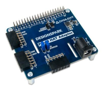
The Pmod HAT Adapter makes it easy to connect Digilent Pmods to a Raspberry Pi. It supports plug-and-play functionality, only requiring that the host Raspberry Pi be booted with the Pmod HAT attached. The Pmod HAT has three 2×6 Digilent Pmod ports and provides access to additional I/O available via the Raspberry Pi 40- pin GPIO connector. The Pmod HAT Adapter comes with example Python libraries hosted on DesignSpark. See the Software Support section below for more information.
