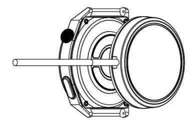
Need to charge and activate before usig the watch for the first time. Use the equipped magnetic wireless charger to attach to The metal ring on the back of the watch, the other charging cable Connect to US8 charging head or USB interface Can
