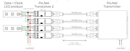
Wiring scheme 6 Combine short & long range Data + Clock SPI
