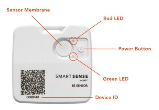
1. Hold the power button for 2-5 seconds, then release to turn on the B3 Sensor.
