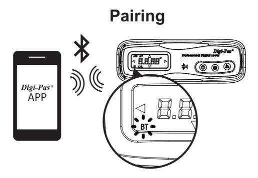
A Press & hold the Power button to power on the digital level. The blinking "BT" indicates the device is waiting to be paired & initialized\*.
