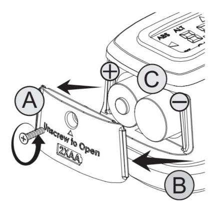
A Loosen screw by turning anti-clockwise direction using a Philips screwdriver B Pull out the battery cap
