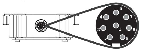
Sensor DB-9 Male cable connector pin-out
