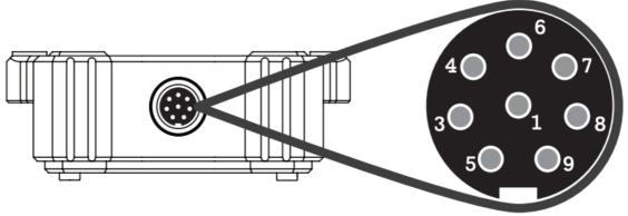
Sensor DB-9 Male cable connector pin-out
