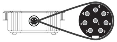
Sensor DB-9 Male cable connector pin-out
