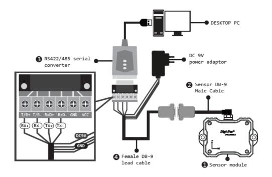
Multiple sensor connection diagram using control box
