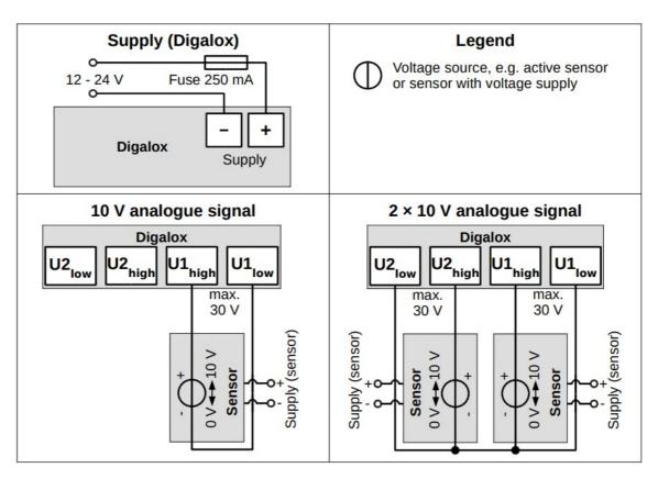
**WARNING:** The device may only be operated in one of the connection options shown above! If two sensors are used, both must be active. If one sensor is inactive, there must not be anything connected to the corresponding low measuring input, otherwise incorrect values will be measured.
