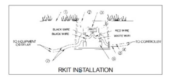
If using a LEIT series controller to switch on a pump, fertilizer injector, fountain or light, there are two connection options using the RKIT 8810. OPTION 1: Install the RKIT to the MV/Pump terminal on the LEIT 4000, LEIT-X and LEIT-XRC controllers. If using the LEIT 4008 use station #8. This will operate all valves with the unit that you are connecting too (e.g. pump).
