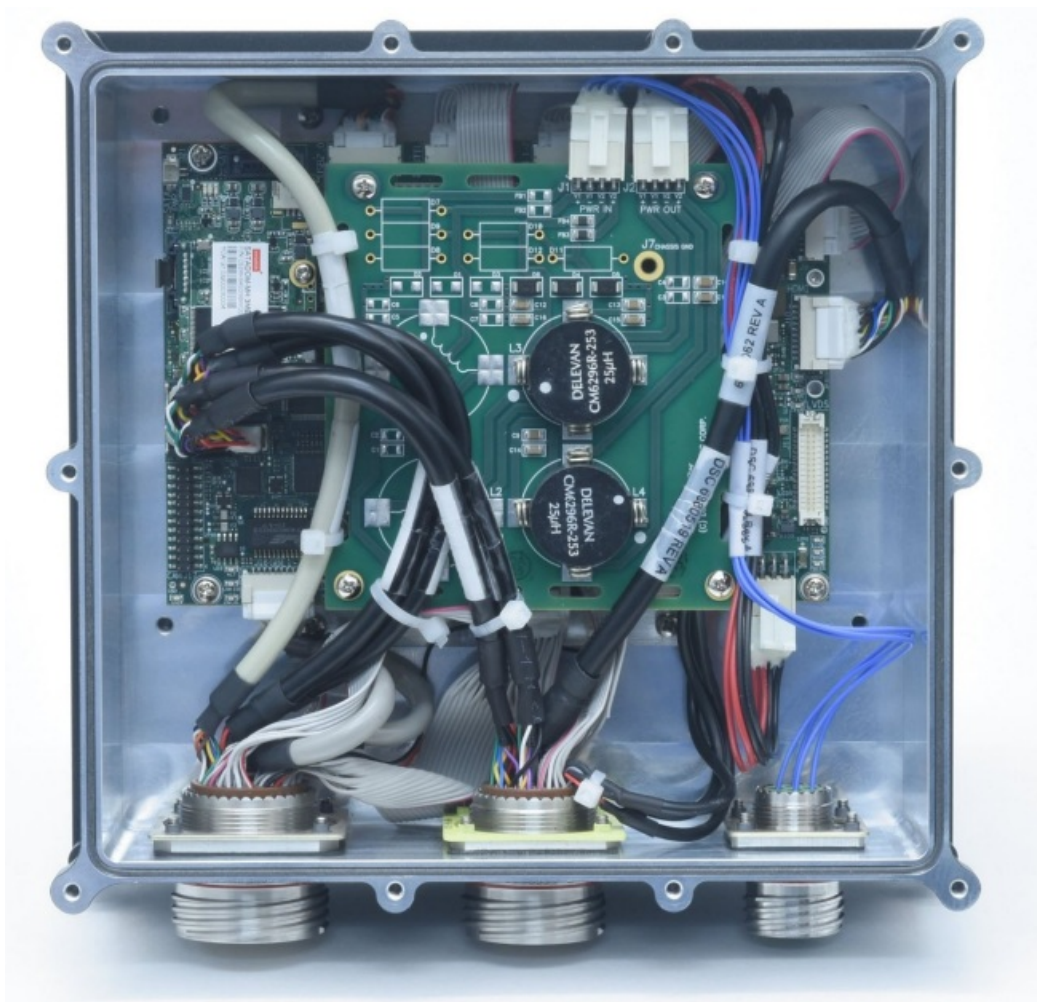
Internal view from bottom of enclosure (bottom cover and JMM-7500 power supply removed)
