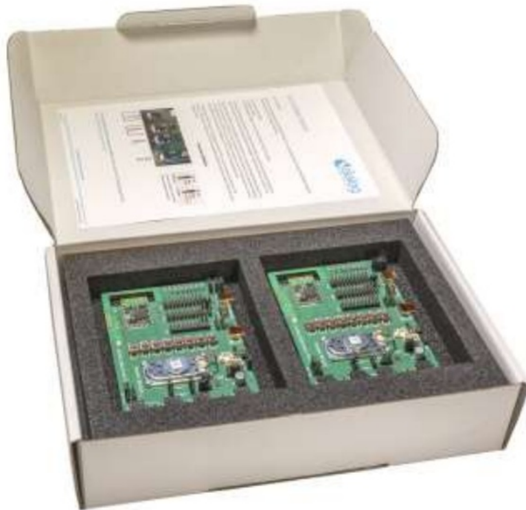
Figure 8: DA14AVDDECTDEVKT with two Carrier Boards
