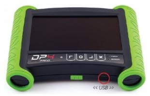
2. DiagProg4 can be updated using the dedicated software DiagProg4 Manager. The device should be connected to an additional power source and connected to the PC via a USB cable. After running DiagProg4 Manager, a desktop with a menu will appear. Select the update/ activation icon and select where to save file (you should select DiagProg4 microSD card).
