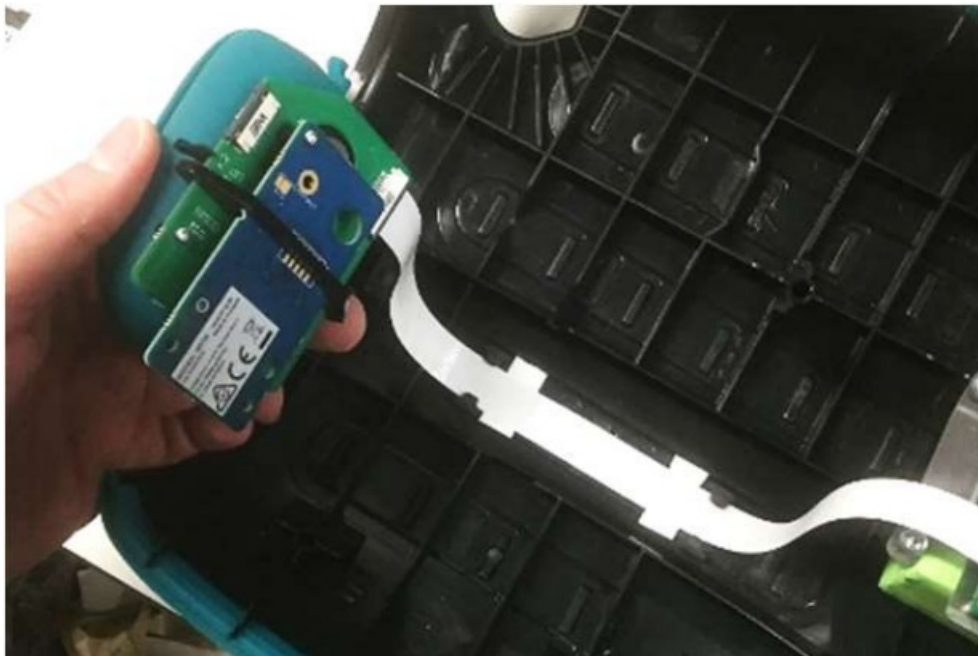
4. Position assembly in side cut-out of lower case
