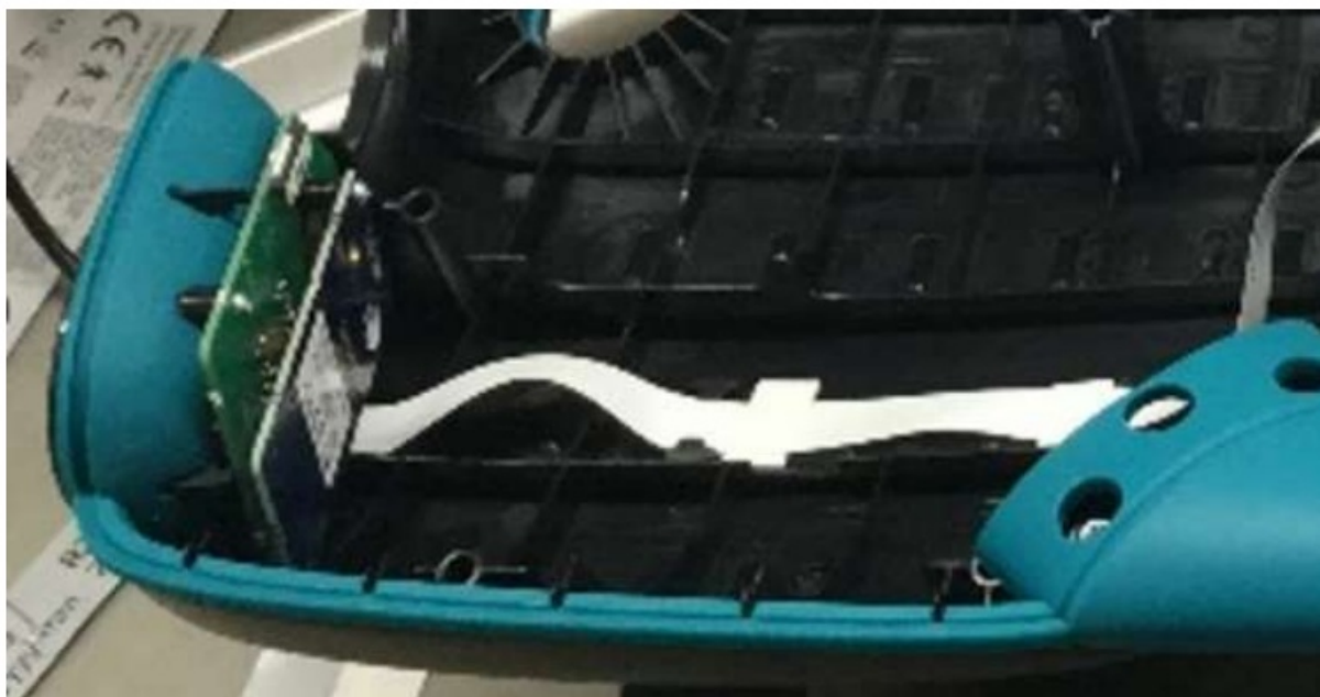
4. Position assembly in side cut-out of lower case
