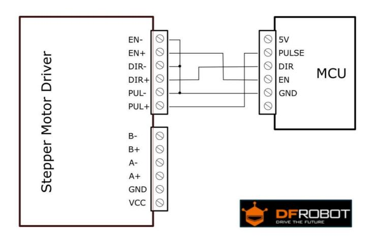
Note: When "EN" is in the valid state, the motor is in a free states (Off-line mode). In this mode, you can adjust the
