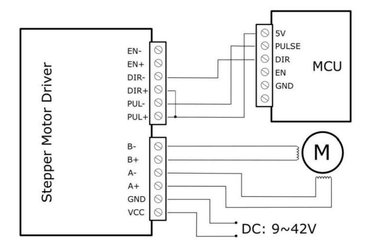
**Note:** Please cut off the power when you connect the system, and ensure the power polar is correct. Or it will damage the controller.
