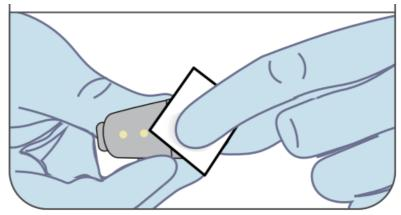
2. Insert transmitter. Only use alcohol tab first, into wipe. holder.
