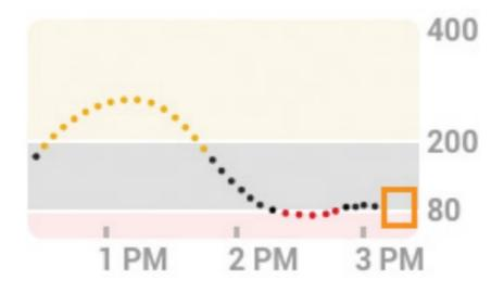
When your G6 Pro readings resume, up to 3 hours of missed readings can fill in on the graph.
