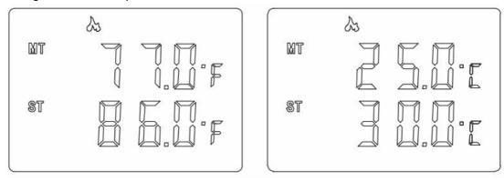
F/°C switch: Press SET button, when "° F" or "°C" flashes, press UP or DOWN Button to switch ° F/°C, wait for 5s, "° F" or "°C" stops flashing, indicating that the switch is successful, the default is ° F.
