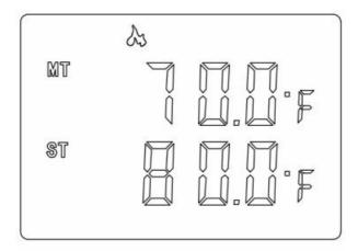
Press the MODE button to switch the heating icon flashing, then press SET button to confirm, the heating
