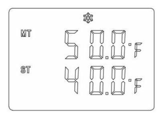
Press the MODE button to switch to the cooling icon: : flashing, then press SET button to confirm, the
