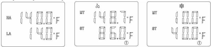
**High Temperature Alarm:** Press SET button, when "HA" flashes, press UP or DOWN Button to adjust the temperature of high temperature alarm in the first line, wait for 5s, "HA" stops flashing, indicating that the setting is successful, and the default HA is 140° F/60°C.
