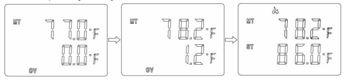
**Calibration Value:** Press SET button, when "CV" flashes, press UP or DOWN Button to adjust the compensation temperature in the second line, the test temperature in the first line follows the change, wait for 5s, "CV" stops flashing, indicating that the setting is successful, and the default CV is 0.0° F/°C.
