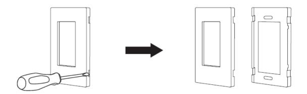
1. Separate the upper and lower shells of the Wall Switch.
