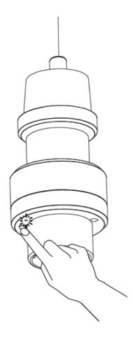
1. Press the program button on the receiver for 3 seconds until the indicator light starts to flash slowly.
