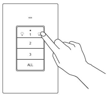
2. Release the program button, then press the ON button (1) on the transmitter, and after 1 second, press the OFF button (1).
