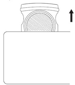
2. Remove the isolation tab in the battery compartment of the transmitter.
