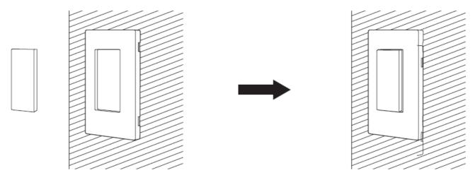
4. Attach the transmitter to the base.
