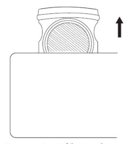
2. Remove the isolation tab in the battery compartment of the transmitter.
