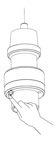
1. Press the program button on the receiver for 3 seconds until the indicator light starts to flash slowly.
