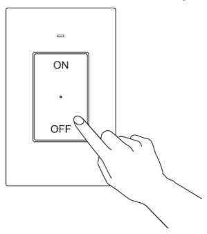
2. Release the program button, then press the ON button (1) on the transmitter, and after 1 second, press the OFF button (1).
