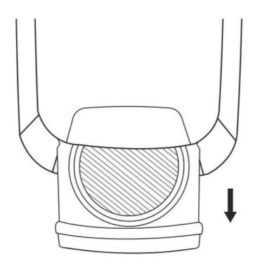
2. Remove the isolation tab in the battery compartment of the transmitter.
