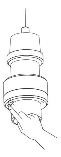
1. Press the program button on the receiver for 6 seconds until the indicator light starts to flash rapidly. (Note: The light flashes from slowly to rapidly.)
