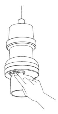
1. Press the program button on the receiver for 3 seconds until the indicator light starts to flash slowly.
