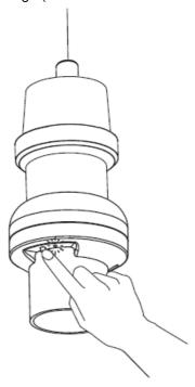
1. Press the program button on the receiver for 6 seconds until the indicator light starts to flash rapidly. (Note: The light flashes from slowly to rapidly.)
