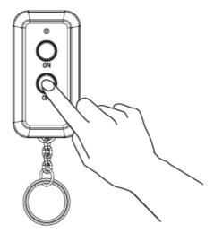
3. Press the ON/OFF button on the wall and switch the remote control to turn the receiver on and off.
