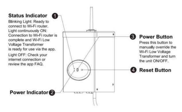
**IMPORTANT:** Please refer to INSTALLATION INSTRUCTION before proceeding with the Wi-Fi router connection. Wi-Fi Low Voltage Transformer must be installed before connecting to the Wi-Fi router.
