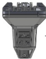
USB-C charging port - power in and power out to charge other devices
