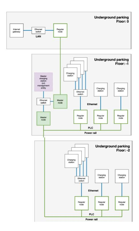
Alternatively, Ethernet cabling can be used to connect several MultiNode networks across floors of the car park as shown below:
