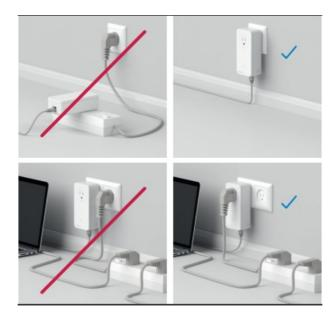
Plug the devolo Magic LAN triple adapter into an available wall outlet and wait until the LED flashes white (approx. 15 seconds).
