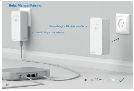
Within 3 minutes, press the button on the side of your devolo Magic LAN adapter, which is connected to the router. Then press the button on your second Magic LAN adapter. When all of the LEDs light up white, pairing has been completed successfully.
