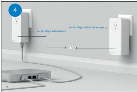
The process is finished when the LEDs on all the devices turn solid white. The process takes a maximum of 3 minutes.
