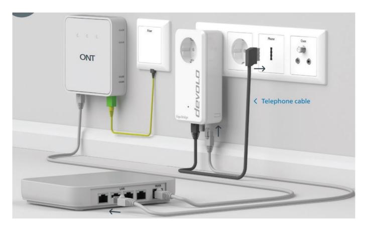
Connect the devolo Giga Bridge adapter to a LAN port (Local Area Network) of the router using the provided
