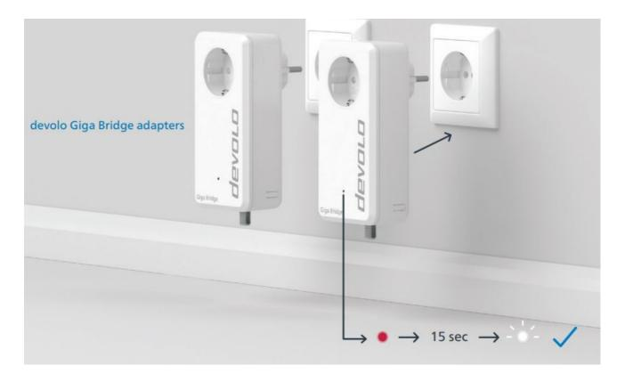
If you have purchased a single adapter to expand your existing network, start the installation with page 9. Otherwise, connect both devolo Giga Bridge adapters to an available power socket. The LEDs of both adapters flash white. Carry out the next installation step within 3 minutes.
