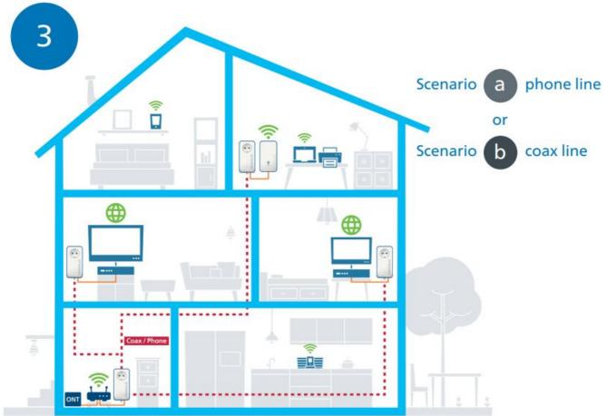
The devolo Giga Bridge uses G.hn technology for the transmission of the Internet signal over coaxial (TV/SAT) or telephone line. In scenario "a" (as of p. 15), the G.hn signal is transmitted over two telephone wires or in scenario "b" (as of p. 19) via standard coaxial cable.
