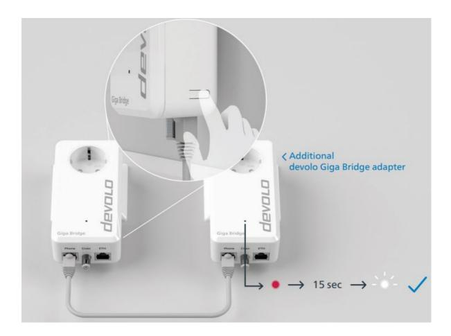
If you want to integrate an additional adapter into your network, plug the additional adapter into a socket next to an adapter that has already been paired. Connect both adapters with the network cable supplied via the phone socket. Press the button on the right edge of the already installed adapter within 2 minutes. The LEDs of both adapters flash white.
