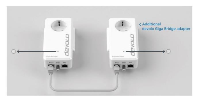
The new adapter is automatically integrated into the devolo Giga Bridge network (pairing). Pairing is complete as soon as the LEDs of both adapters light up white continuously. You can remove the network cable and plug in the adapters where you want to use them. Go to p. 17 (Phone) or p. 21 (Coax).
