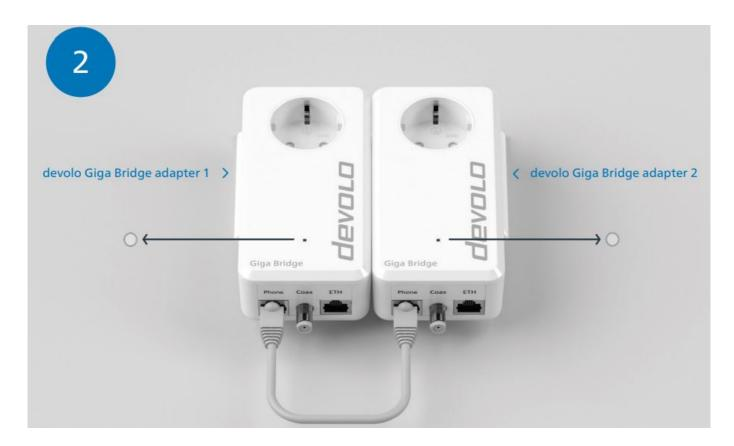
Connect the two devolo Giga Bridge adapters to the phone sockets using the network cable supplied. A new devolo Giga Bridge network is automatically set up (pairing). When both LEDs light up white continuously, the process is complete and you can remove the network cable again.
