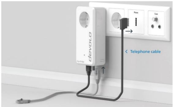
Now place the additional Giga Bridge adapter(s) in the preferred rooms. Connect the devolo Giga Bridge adapter to the wall connection using the provided telephone cable. You can then connect your end devices or Wi-Fi access points via an Ethernet cable. Done.
