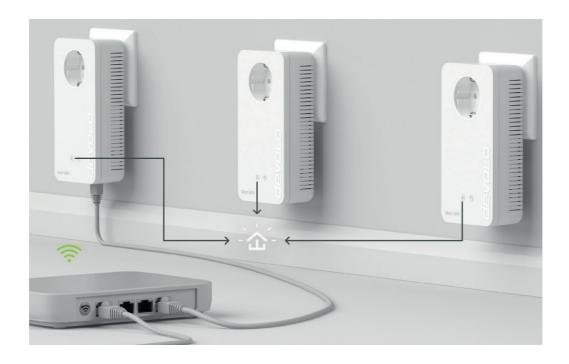
The encryption process takes place automatically. During this time, the LEDs of all adapters will flash white.
