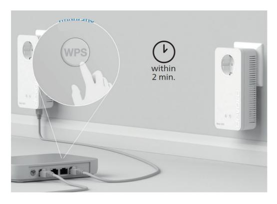
Within 2 minutes, press the WPS button on your Wi-Fi router. If necessary, please refer to the manual for your router to find the location of the WPS button and how long you have to press it.
