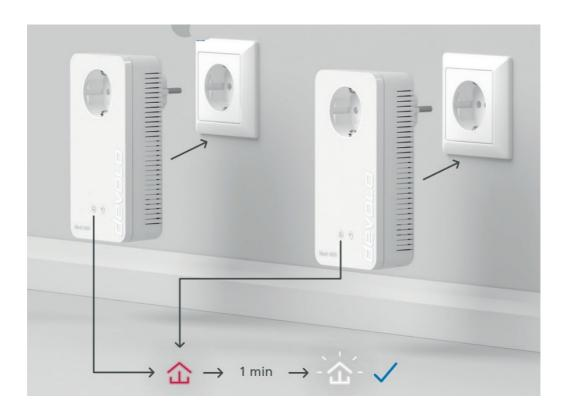
**Help:** If pairing during initial installation was unsuccessful, you can carry out the manual pairing of the adapters. Connect the devolo adapters to a free wall socket and wait until the LED lashes white (approx. 1 min.).
