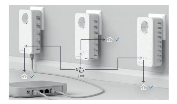
Press the button on all devolo adapters within 3 minutes. Once all LEDs light up white, the pairing has been completed successfully.
