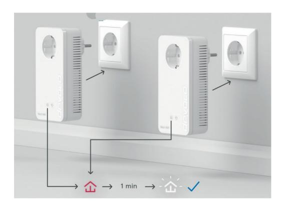
Plug two of the adapters into an available power socket and wait until the LED flashes white quickly (about 1 min.).
