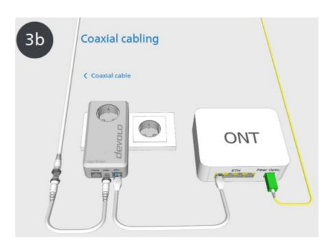
Connect the devolo Giga Bridge adapter to the existing coaxial cabling. To do this, use the provided cable and connect it to the coaxial socket (Coax) of the Giga Bridge. Connect the devolo Giga Bridge to the NT/ONT-Box using the provided network cable.
