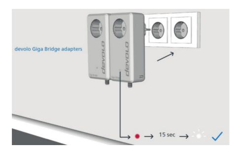
Connect both develop Giga Bridge adapters to an available power socket. The LEDs of both adapters flash white. Carry out the next installation step within 3 minutes.
