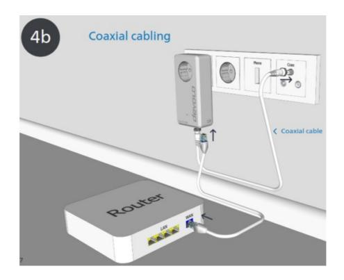
Connect the second devolo Giga Bridge adapter to the WAN (Wide Area Network) port of the router using the provided network cable. Connect the devolo Giga Bridge to an existing connection in the wall via the F-type socket (Coax). Done!
