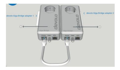
Connect the two devolo Giga Bridge adapters to the phone sockets using the network cable supplied. A new devolo Giga Bridge network is automatically set up (pairing).
