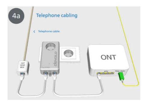
Connect the devolo Giga Bridge adapter to the existing wall connection (CAT RJ 45 box) via the phone socket. Use the provided telephone cable for this purpose. Now connect the devolo Giga Bridge to the NT/ONT-Box using the provided network cable.
