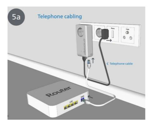
Connect the second devolo Giga Bridge adapter to the WAN (Wide Area Network) port of the router using the provided network cable. Now use the telephone cable to connect the devolo Giga Bridge (Phone socket) to the wall connection. Done!
