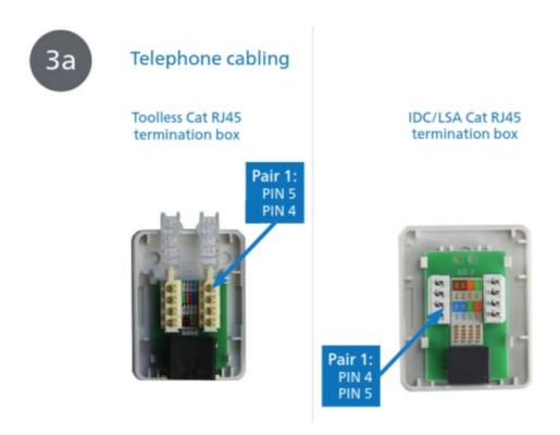
The telephone cable is removed from the demarcation point and then split and secured by means of connection technology involving wire stripping and soldering or screwing down. A standard network interface is created as a result.
