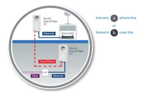
The devolo Giga Bridge uses G.hn technology for the transmission of the Internet signal over coaxial (TV/SAT) or telephone line. In scenario "a" (as of p. 9), the G.hn signal is transmitted over two telephone wires or in scenario "b" (as of p. 15) via standard coaxial cable.
