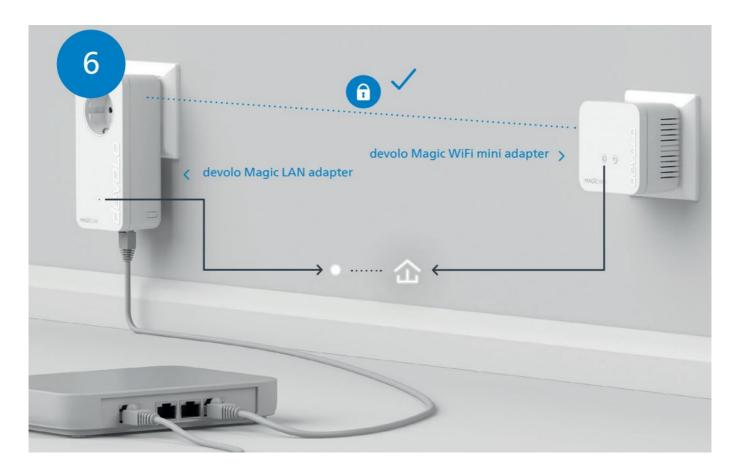
Set up the Wi-Fi connection on your smartphone, etc. The basic installation process is complete. If you have not so far had a Magic WiFi adapter on your network, you can subsequently and optionally set up Mesh Wi-Fi technology.
