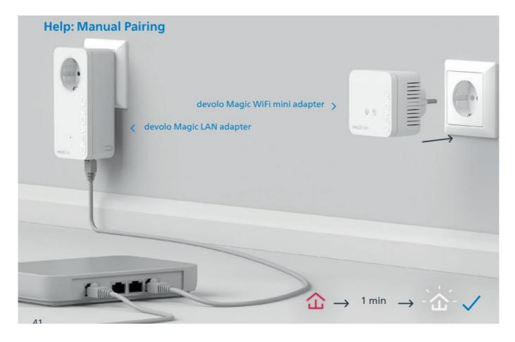
Help: If automatic pairing during initial installation was unsuccessful, you can carry out manual pairing of the Magic adapters. Connect the devolo Magic WiFi mini adapter to a free wall socket and wait until the LED flashes white (approx. 1 minute)
