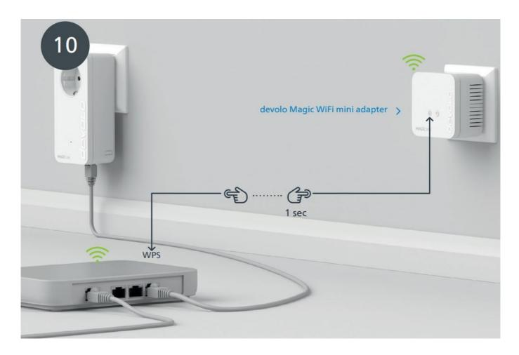
Once the LED lights up solid white, the process has been completed successfully.
