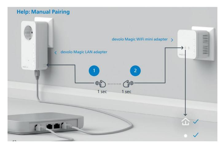
Within 3 minutes, press the button on the side of your devolo Magic LAN adapter which is connected to the router. Second, press the LED on your Magic WiFi mini adapter. As soon as all of the LEDs light up white, pairing has
