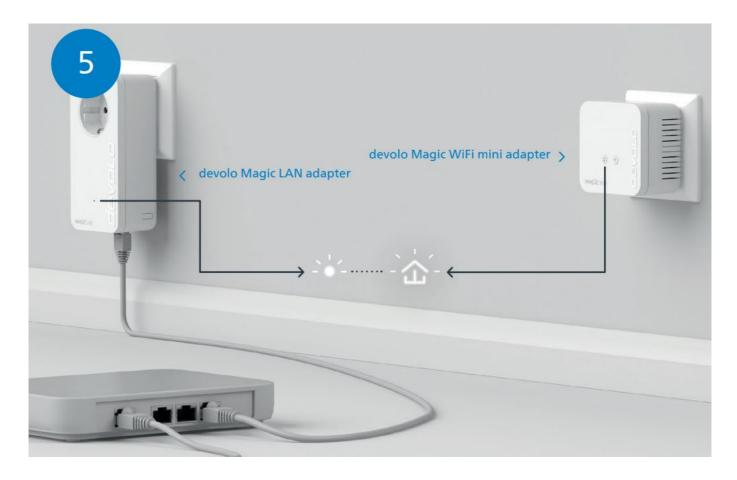
The process is complete as soon as all of the LEDs on the devices light up solid white. The process takes a maximum of 3 minutes.
