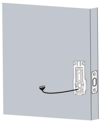
3. Secure the back cover with screws.
