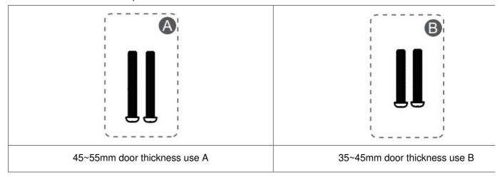
4. Tightly fasten the screws in place. Set the screws with your hands, then use a screwdriver to secure them.
