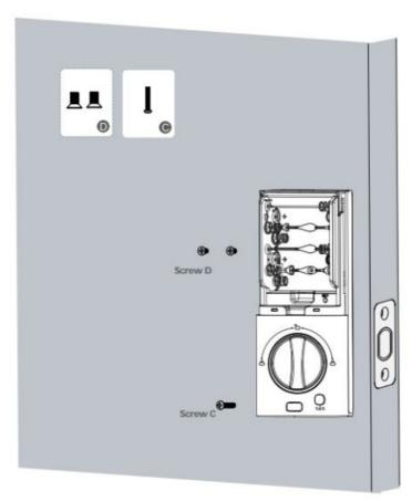
9. Install 8 AA batteries into the door lock and it is ready to be used.
