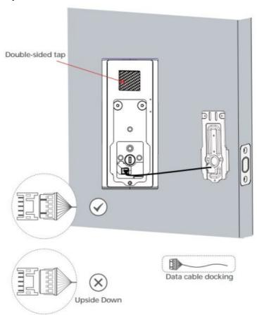
7. Mount the interior assembly. Make sure the wire is tucked into the cabin on the back of the interior assembly.
