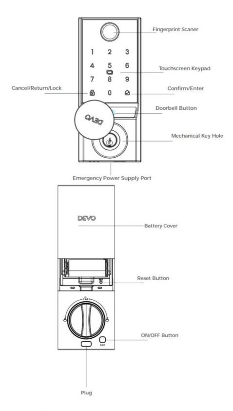
**Notes:** The "Emergency Power Supply Port" is not for battery charging purpose and can only be used for emergency power supply to the lock.
