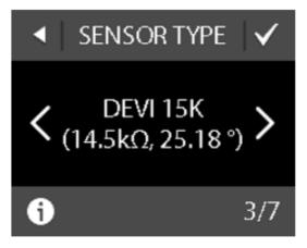
8. Use the < and > arrows to select the installed floor sensor type. (Measured resistance and corresponding temperature are shown in brackets). Press to confirm.
