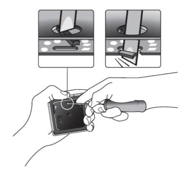
If you break the small plastic seal on the back of the display module, e.g. using a screwdriver, it will be possible to set the maximum floor temperature up to 45°. Furthermore, it will be possible to use only a room sensor. However, this option is not recommendable due to an increased risk of overheating the floor.
