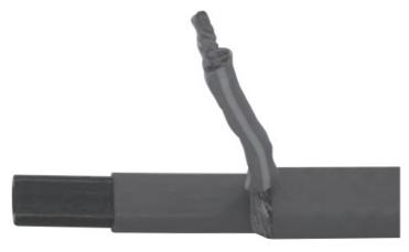
4. Cut into the heating element, bend it and pull it off the wire strands using fiat nose pliers. Twisting stranded wires
