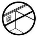
• The thermostat must not be installed in direct wet areas (Zones 0, 1, and 2). Always follow local regulations regarding IP classes, this doesn't mean that the thermostats can't be installed in bathrooms.
