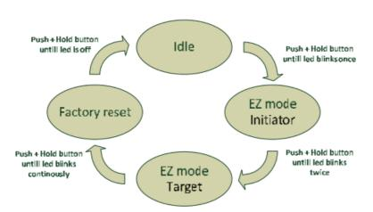
When cycling through the menu modes, the state is indicated by a number of 100ms blinks on the LED. The device is supporting the ZigBee standardized EZ- mode Commissioning.
