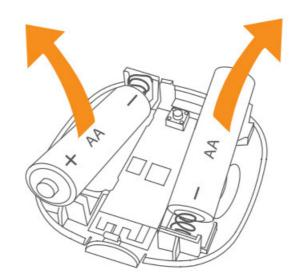
2. Replace the batteries respecting the polarities.
