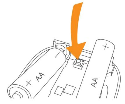
3. While you are holding the button down, the LED first flashes once, then two times in a row, and finally
