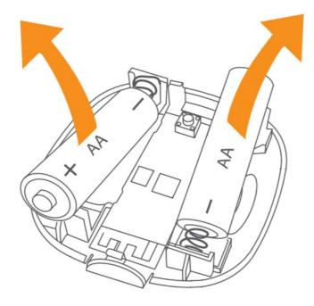
2. Replace the batteries respecting the polarities.
