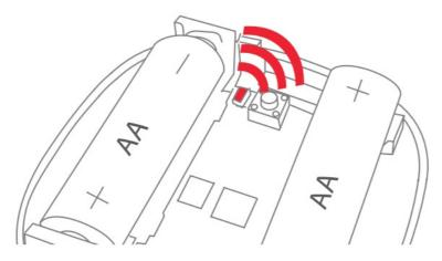
6. When the LED stops flashing, the Humidity Sensor has successfully joined the ZigBee network.
