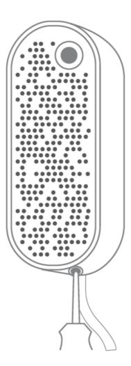
2. Use the included screws to mount the range extender on the wall.
