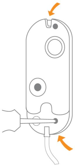
3. Attach the front cover to the device by hooking the front cover to the top of the mounted device and pushing the front cover against the device.
