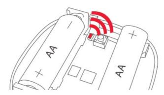
6. When the LED stops flashing, the Smart Humidity Sensor has successfully joined the Zigbee network.
