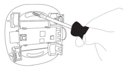
3. Insert batteries respecting the polarities.
