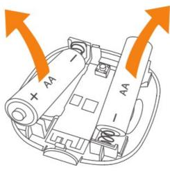
2. Replace the batteries respecting the polarities.
