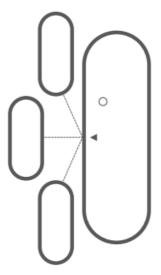
• The sensor and magnet may be placed on separate three dimensional planes, though this does affect the maximum distance allowed. The magnet may also be placed either facing the side of the sensor or sitting parallel to it.
