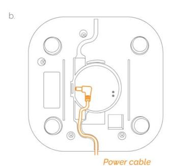
3. Place the device on top of the wall bracket and slide it down until it clicks.
