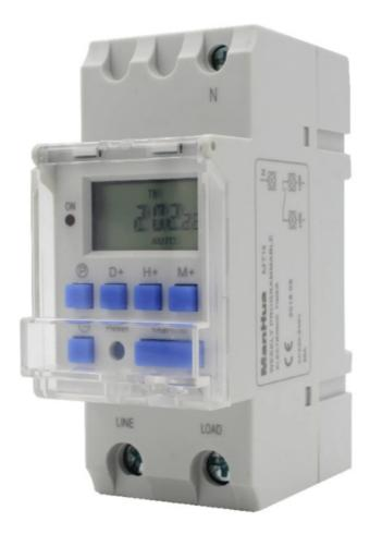
The PTM seven day timer allows for the programming of open and close times for overhead doors, gates and parking barriers. It is designed with 16 ON/OFF events per day and 15 combinations of daily programs for the best flexibility to the user. This DIN rail mounted timer has an internal battery for memory back-up in the event of a power failure.
