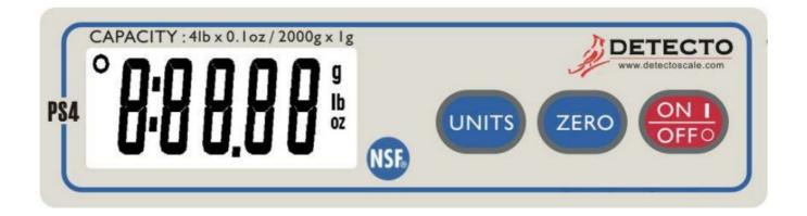
The annunciators are turned on to indicate that the scale display is in the mode corresponding to the annunciator label or that the status indicated by the label is active.
